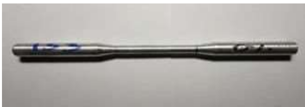
Fig.4: Prepared tensile test specimen
